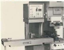
This is a microcomputer-controlled X-Y positioning system. Memory capacity is 99 programs of 120 steps each. When press power is turned off, an internal battery maintains the programs intact.
