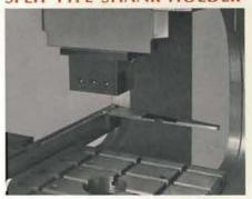
A Shank Holder enables the SPH to be used as a stamping press, using exising tools.
