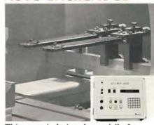
This gauge is designed especially for bending operations. It is controlled by key board with LED display, and can store 50 different bending positions.
